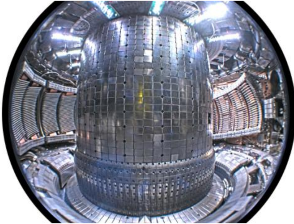
Interior of Alcator C-Mod showing the molybdenum tiles used as first wall material
