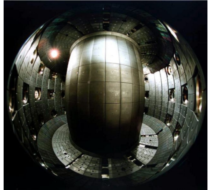
Interior of Tokamak à configuration variable showing the graphite tiles used as first wall material
